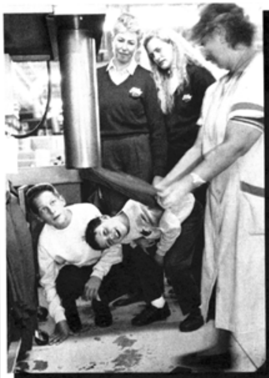
How does it do that? Jonathan and Andrew take a closer look at the powerful vacuum machine as it instantly flips a completed pair of trousers right side out ready for pressing and sucks away any lint, loose thread, and other fluff.
