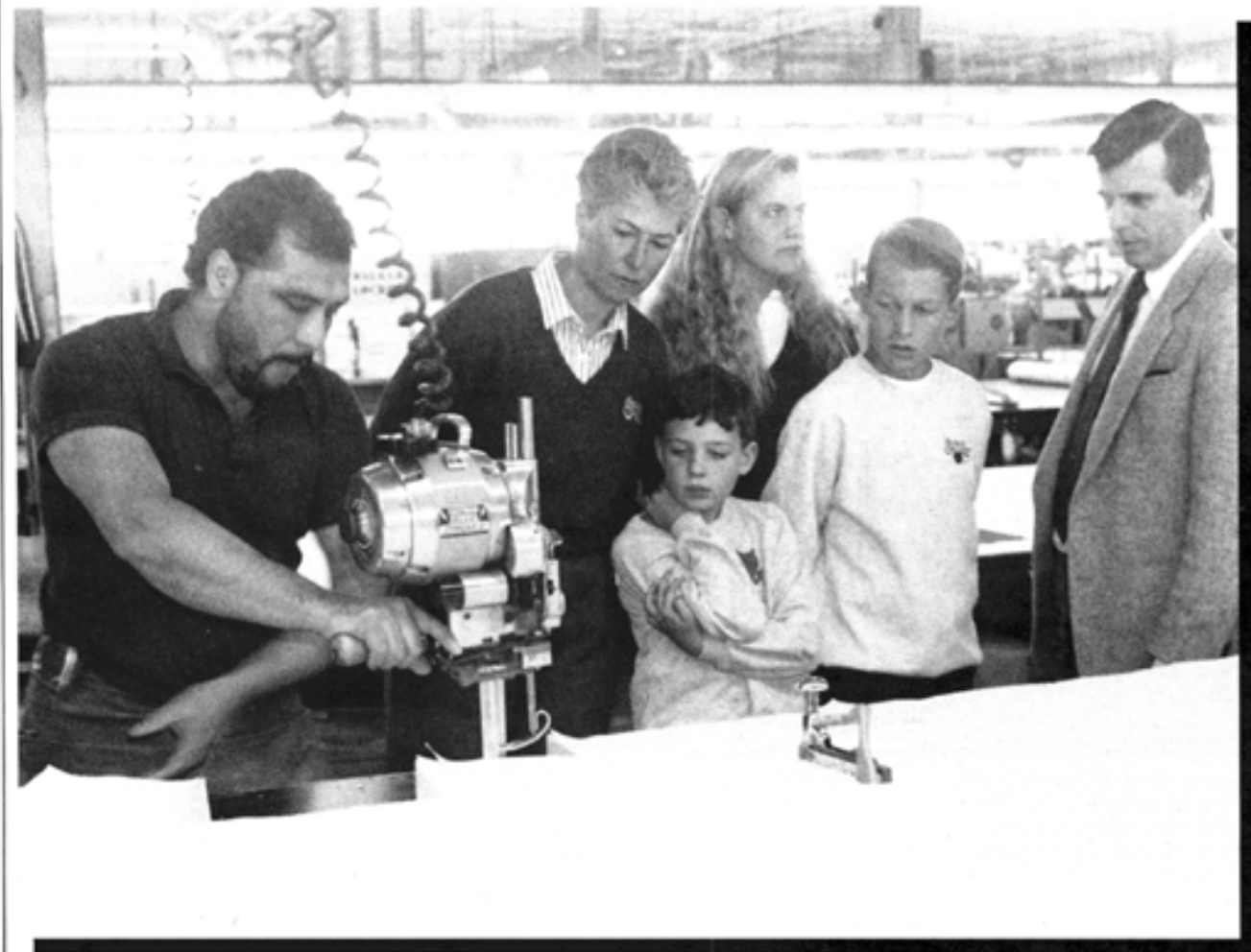
Andrew keeps his fingers well out of the way as a cutting table operator cuts around a Scout shirt pattern piece. The blade slices through more than 10 cm of fabric as quickly and easily as if it were slicing room-temperature butter. Jim Petrie, right, says operators can cut out as many as 200 pieces at a time.
